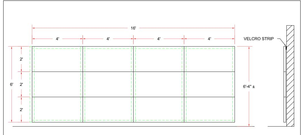
\_\_\_\_\_ SECTIONS OF WALL PADDING 16' WIDE x 6' HIGH CONSISTING OF FOUR (4) 4' x 6' TRI-FOLDING ALL PURPOSE PADS WITH VELCRO ON ALL 4 SIDES STANDARD FOLD, 2' PANELS AND HUNG WITH RS GMH - ALUMINUM GYM MAT HANGER AND VELCRO.
